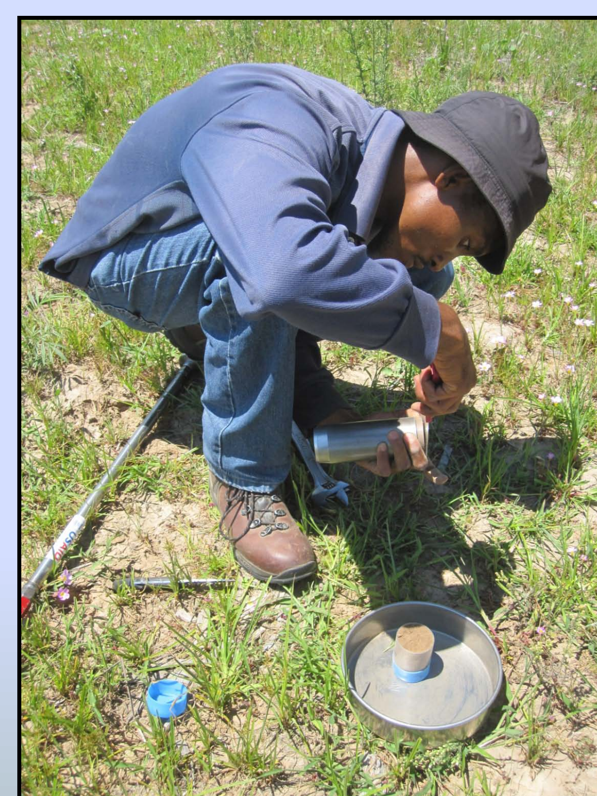
Collecting bulk density samples in Roma, Lesotho.
