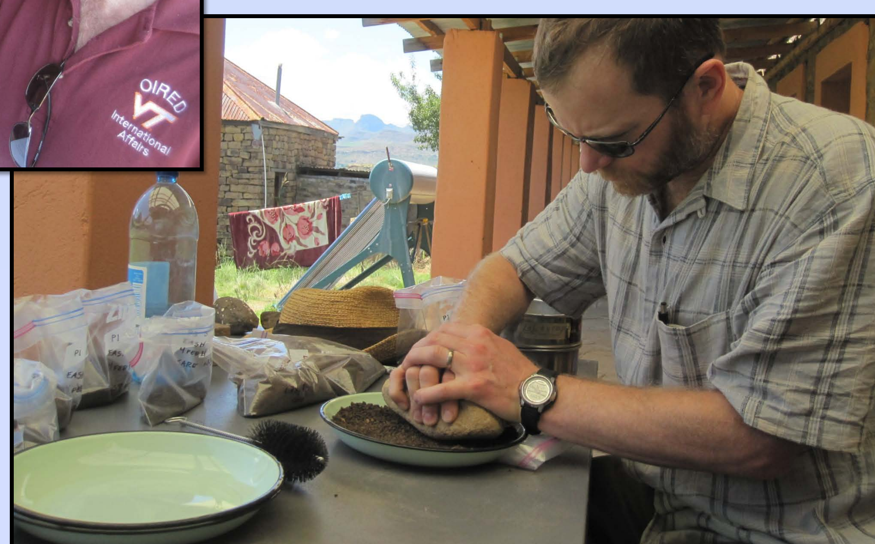
Grinding soil samples to pass a 2 mm sieve for shipping in Matphutseng, Lesotho.
